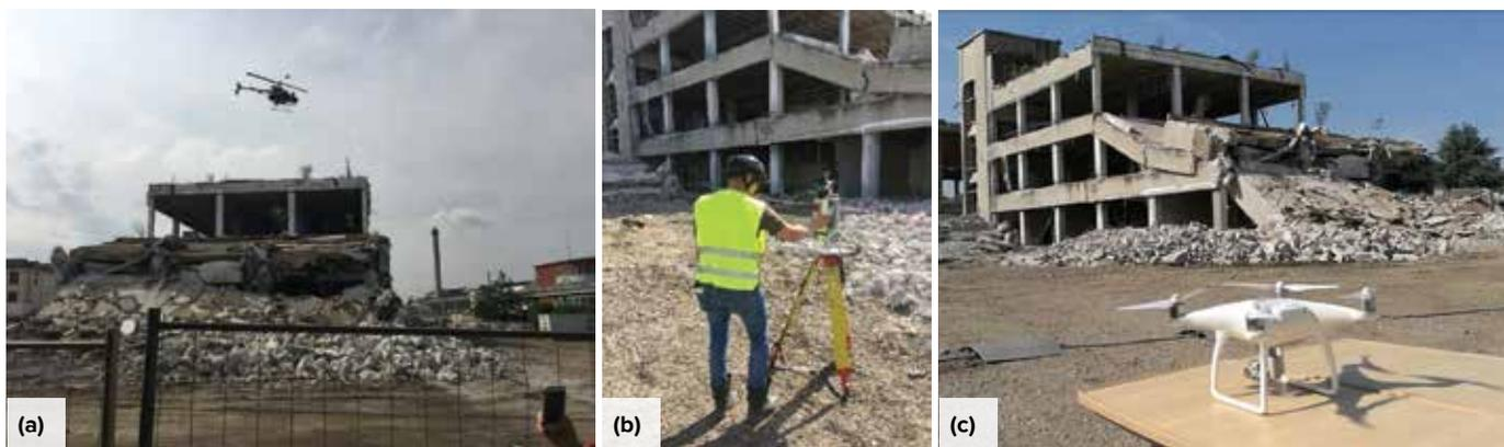
**Fig. 1:** INACHUS tools applied during the second field test included: (a) a UAV with a laser scanner; (b) a ground-based laser scanner; and (c) a UAV with a digital optical camera (photos courtesy of INACHUS project)
